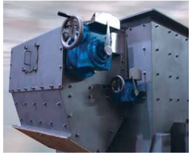
Adjustable bed level and underflow gate
