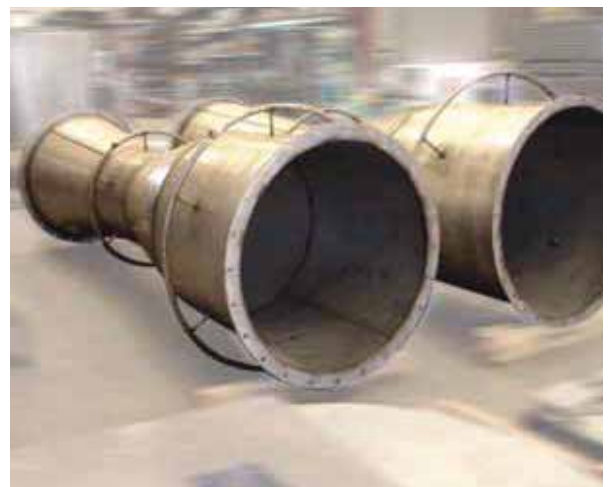
In-duct venturis for continuous flow measurement and control
