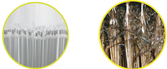
End-Free Fibers Prevent Fouling
