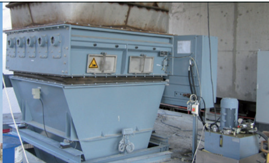
ACQUISITION OF THE EXACT TRANSFER AMOUNT VIA DIFFERENTIAL DOSAGE SCALE. The transfer occurs from the OSZILLOMAT with a great output. Materials: Synthetic gypsum with big stones. Place: Serbia
