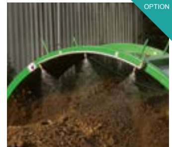
Water sprayer with nozzles. To achieve an optimal microorganism climate within the mound, the addition of water is essential.
